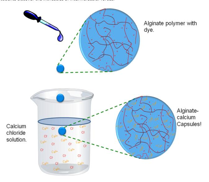
Students then discover the kinetics of the release rates of the dye in the capsules they have made using the UV/Vis Spectrophotometer. Remember, a *supernatant* is the liquid floating on the surface above the solid or precipitate. Absorbance indicates release rate (kinetic activity) of the capsules.
